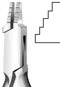
RS-12-6612 Loop Closing Plier, Nance Style Box joint with 4 sectioned tip for forming various size loops in rectangular and round wires. For wires up to .028" ( 0.71 mm).
